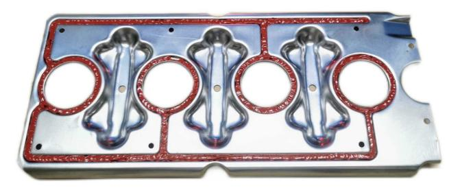
• Mount back the oil baffle with the screws that came of or use screws like below for better grip when removing. Use Loctite to secure the new screws.
