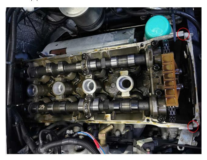
• Now install the valve cover and tighten the valve cover bolts with 3.6Nm when using a silicone gasket in order as below.
