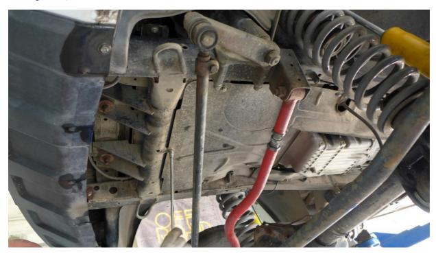
In some cases, it is possible to install the clamp without modifying the protection. Install the bracket corner on the right side of the car frame using a clamp. The ear should be placed outside the car frame and turned downwards. Tighten the clamp nuts after final installation.
