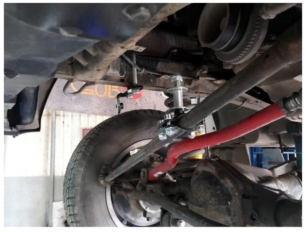
2. Install the finger bracket on the long steering rod. The axis on the bracket is tilted in relation to the axis of the steering rod. The finger should be positioned vertically to the top and have an inclination to the left wheel of the car. The distance between the axes of the brackets is 610-620 mm. Tighten the bracket bolts after final installation.
