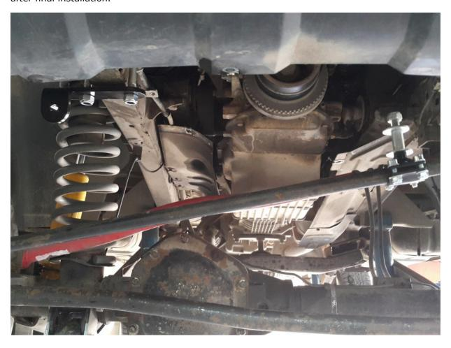
3. Before installing the steering damper, it is necessary to pump it, squeeze it several times , and then unclench it. For installation, it is necessary to set the distance between the axes of the damper 610-620 mm, the wheels of the car should be located in a straight line.
