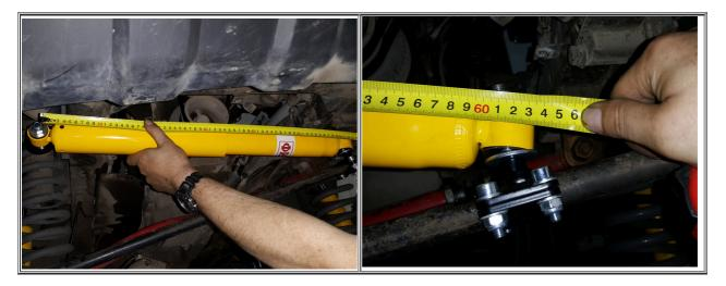
4. The damper should be located directly above the steering rod, along it. The damper cover must be located on the frame bracket.
