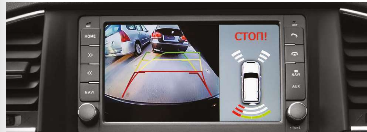
When reversing, a color display shows the view from the rear camera with dynamic guiding lines, and front and rear parking sensor signals
