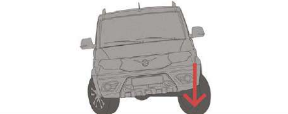
Cornering Brake Control (CBC) distributes braking forces across the wheels when braking on turns
