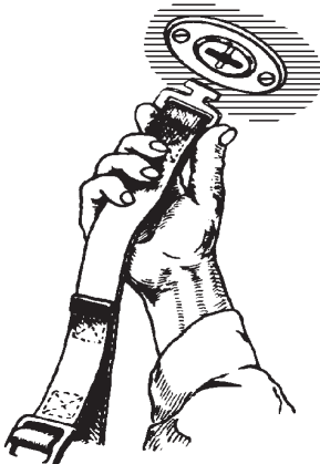
Fig. 3.12. Hanging belt installation
