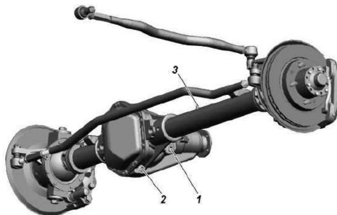
Fig. 9.17 Front axle with a one-piece crankcase:
