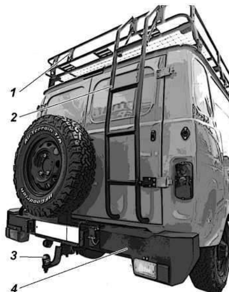
Fig.10.4 Expedition rack on the roof with a ladder 1 - expeditionary rack; 2 - ladder; 3 - pulling device; 4 - rear power metal bumper
