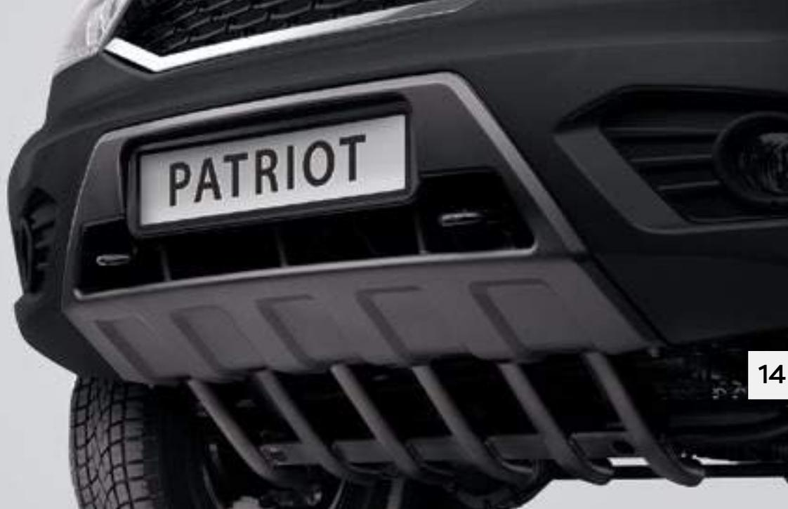
Critical parts of the vehicle demand solid protection, because collisions with obstacles are part of the very nature of the powerful UAZ Patriot. The transmission, transfer case, steering rods and fuel tank should all be well protected. The protection of steering rods is necessary for their safety and proper operation when encountering rough terrain and obstacles. We offer two types of protection: steel pipe or sheet steel skid plates.
